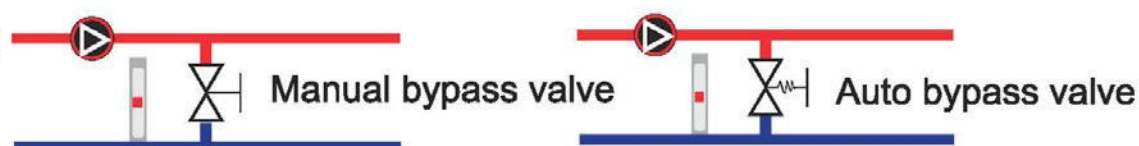
Figure 10 - System installed with bypass valve
